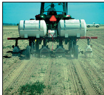
Figure 10. Weed-seeker sprayer, fitted with hood, applying Roundup only to green weeds.
