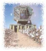
mechanical brushes that remove the entire boll from the plant. In the rest of the Belt, spindle pickers are used. These cotton pickers pull the cotton from the open bolls using revolving barbed spindles that entwine the fiber and release it after it has separated from the boll.
