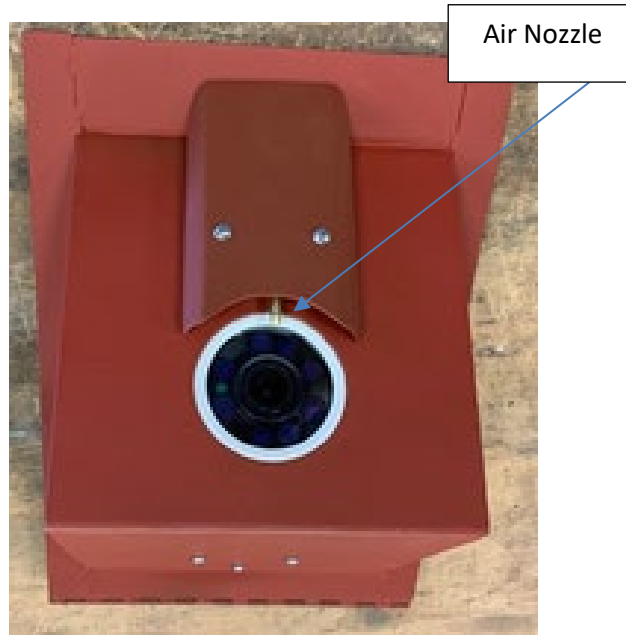
Figure 3. Shows the camera side of the air-inlet tube, back-side view is detailed in Figure 2a, that directs air across the optics thereby providing an air-wash to help keep the optics clean.
