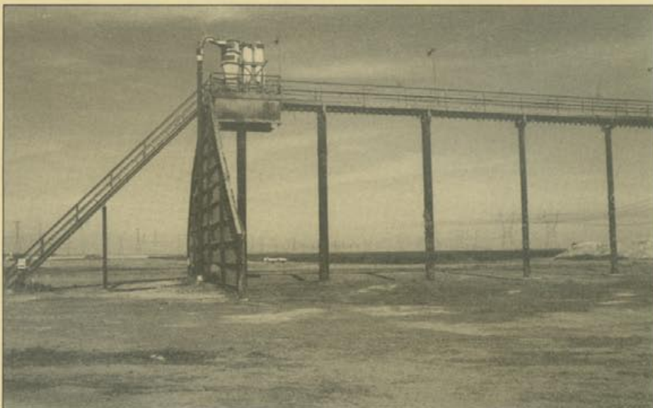
Figure 3. Elevated auger used to drop trash into a pile at the gin.
