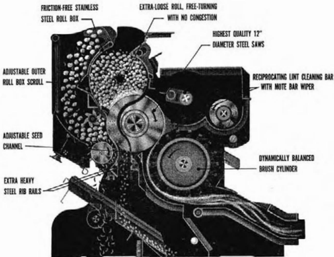
Figure.11. Murray 120 Saw Safety Brush-type Gin.
