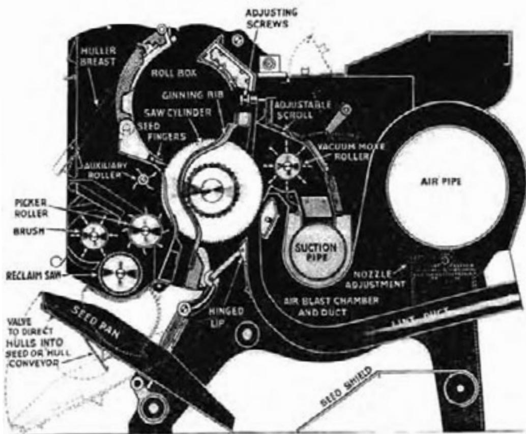
Figure 5. Hardwicke-Etter CXX 120 Saw Air-blast Gin.
