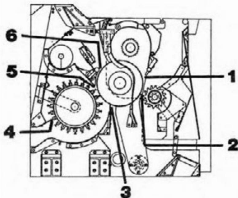
Figure 26. Consolidated Cotton Gin Company, Inc. 112- and 164-saw brush-type Gin. Important noted settings and adjustments are given in the text.
