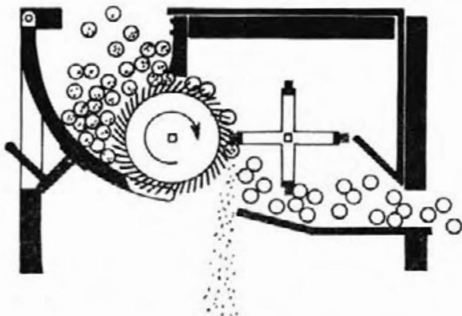
Figure 3. Cross-section of Whitney-type Gin.
