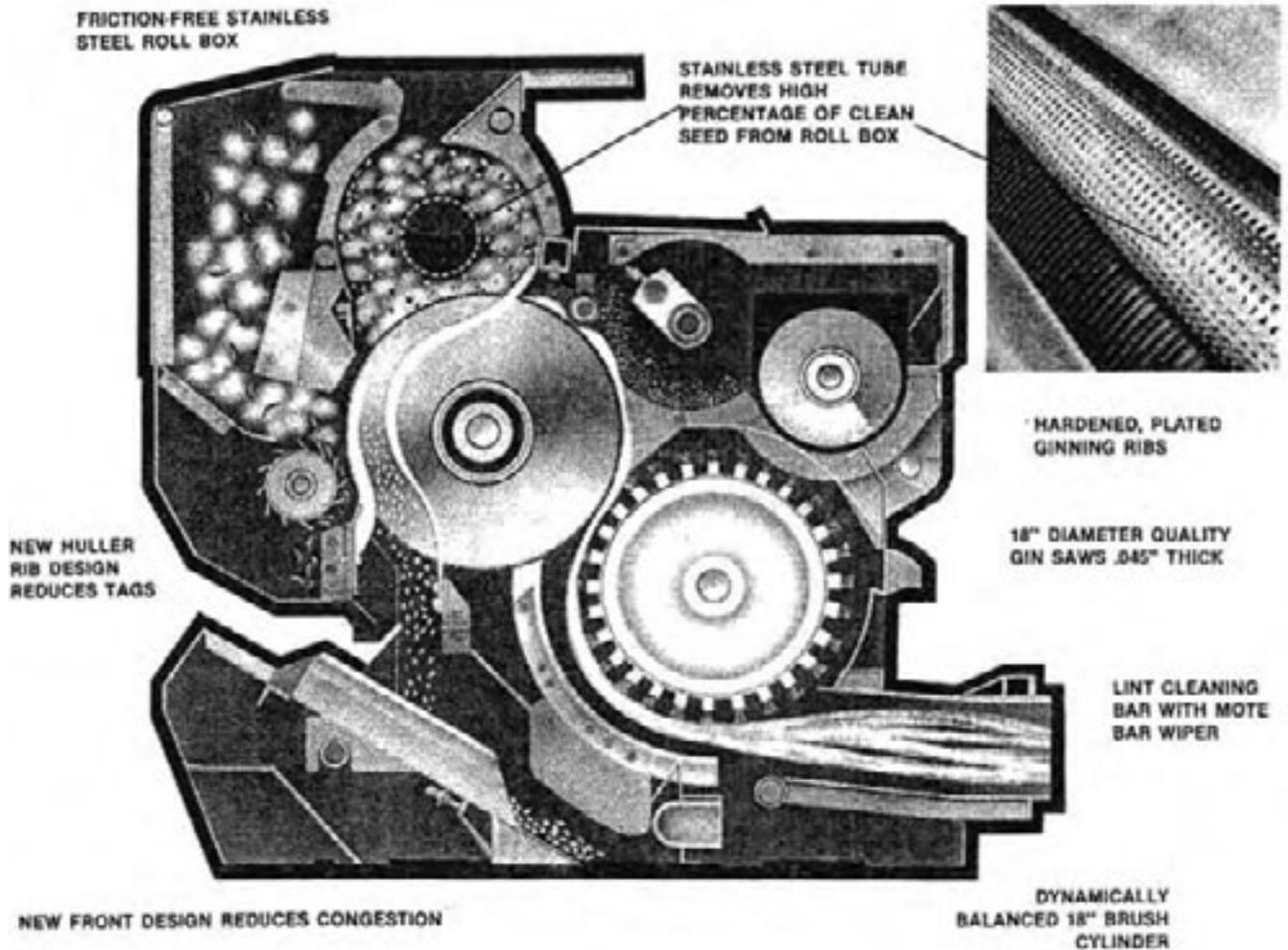
Figure 14. Murray Triple Crown 94/142 Saw Brush Gin.
