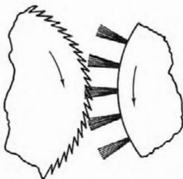
Figure 29. For proper doffing, the gin brush should be set to mesh with the depth of the sawteeth.
