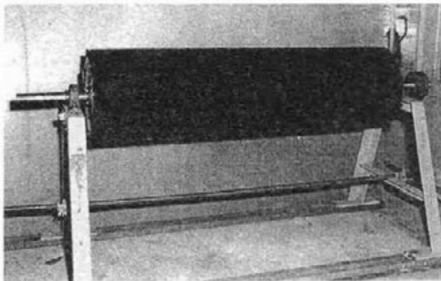
Figure 31. Brush cylinder with a solid doffing surface used to reduce noise.
