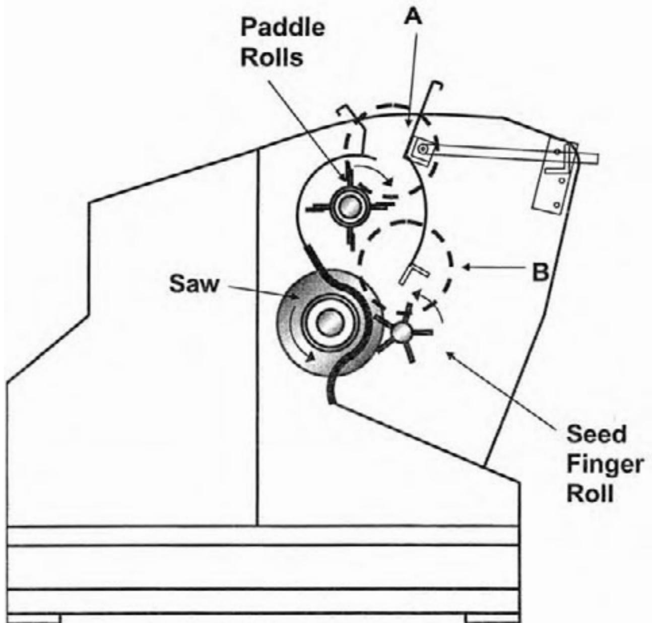
Figure 30. Schematic cross section of Powered Paddle Roll Gin Stand. Circled areas A and B required major changes from the conventional layout.
