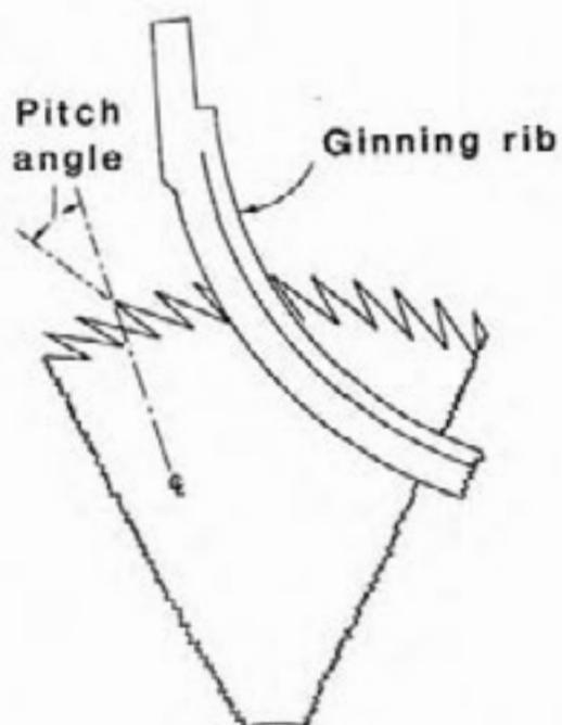
Figure 28. Leading edge of the tooth should enter the ginning rib surface, or the point of the tooth should lead the throat slightly.
