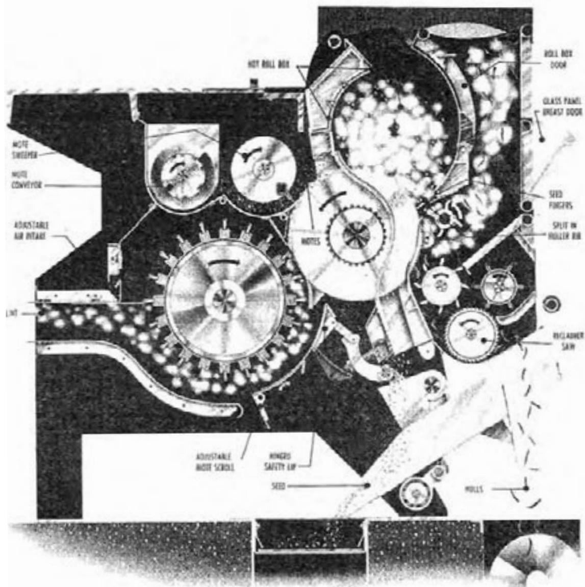
Figure 6. Hardwicke-Etter 100 and 120 Saw Brush-type Gin.
