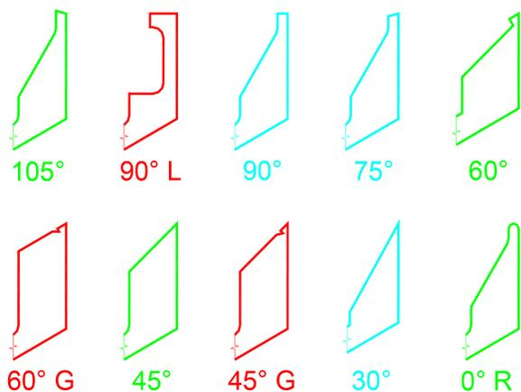
Figure 24. Experimental grid bars (Armijo et al., 2011).
