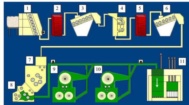
Figure 22. Typical ginning machinery for spindle-picked upland cotton includes a module feeder (1) followed by first stage dryer (2), first cylinder cleaner (3), stick machine (4), second stage dryer (5), second cylinder cleaner (6), extractor-feeder (7), gin stand (8), one or two lint cleaners (9,10), and bale press (11) (Boykin and Ray, 2010).
