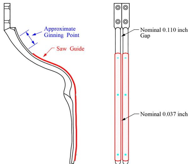
Figure 11. Experimental gin rib and saw guide (Hughs, 2002).
