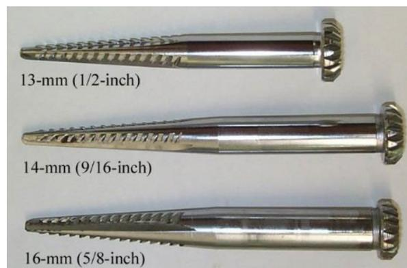
Figure 13. View of 13-mm (0.5 in.), 14-mm (0.56 in., used in another study), and 16-mm (0.63 in.) diameter spindles (Armijo et al., 2006b).
