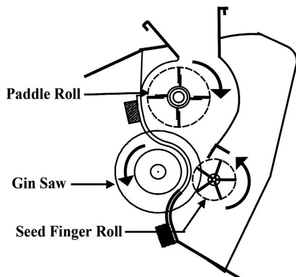
Figure 16. Saw gin stand with paddle-roll seed roll box (Armijo et al. 2006b).
