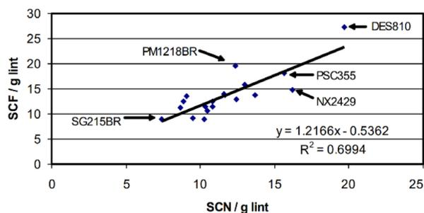
Figure 17. The number of seed coat fragments (manually counted) plotted with the number of seed coat neps determined with the AFIS for cultivars averaged across the three test groups (Boykin, 2008a).
