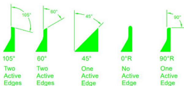
**Figure 26.** Cross-section of the five experimental grid bars used in the study (Armijo et al., 2011).
