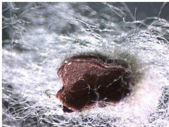
**Figure 1.** Seedcoat fragments (SCF) from the chalazal end of the seed breaking off during ginning. An example of SCF generated during the ginning process.
