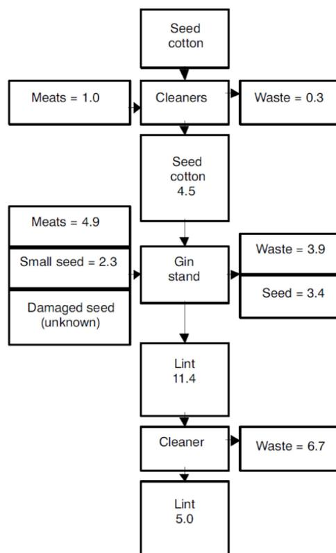
Figure 19. Flowchart showing the origin, content, and removal of seed coat fragments (SCF) in a cotton gin. Units for all numbers are mg SCF per g lint (Boykin, 2008b).
