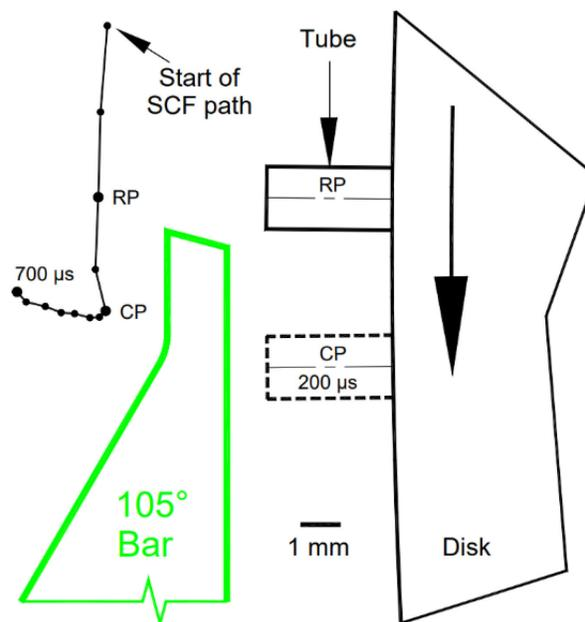
Figure 25. Grid bar: 105°. The distance from the toe to the 2nd corner is 1.55 mm (0.061 in). The seed coat fragment was removed on the second corner (Armijo et al., 2011).
