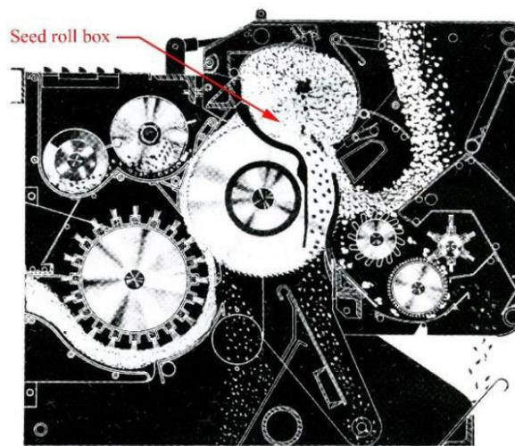
Figure 14. Saw gin stand with traditional seed roll box (Armijo et al., 2006b).
