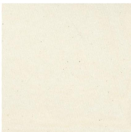
**Figure 28.** Greige fabric knit from test bale sample (dark spots are seed coat fragments).
