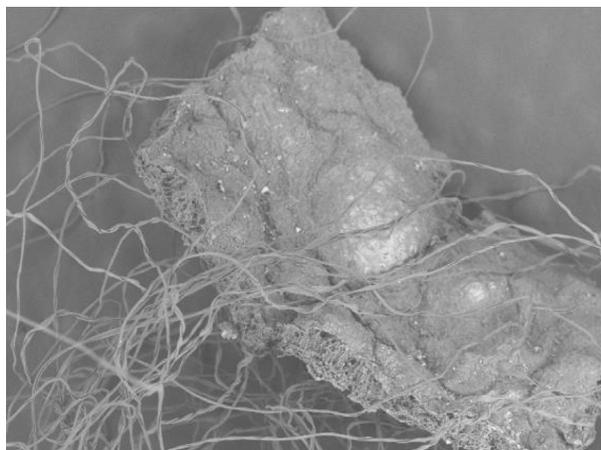
**Figure 3. Seed coat fragment with fibers attached (Fiber and Biopolymer Research Institute, Texas Tech University).**
