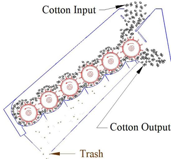
Figure 20. Six-cylinder seed cotton cleaner (Armijo et al., 2009).
