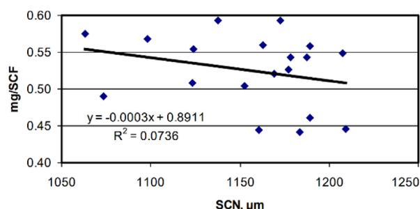
Figure 18. The average weight of individual seed coat fragments (manually fractionated) plotted with the average seed coat nep size determined with the AFIS for cultivars averaged across the three test groups (Boykin, 2008a).
