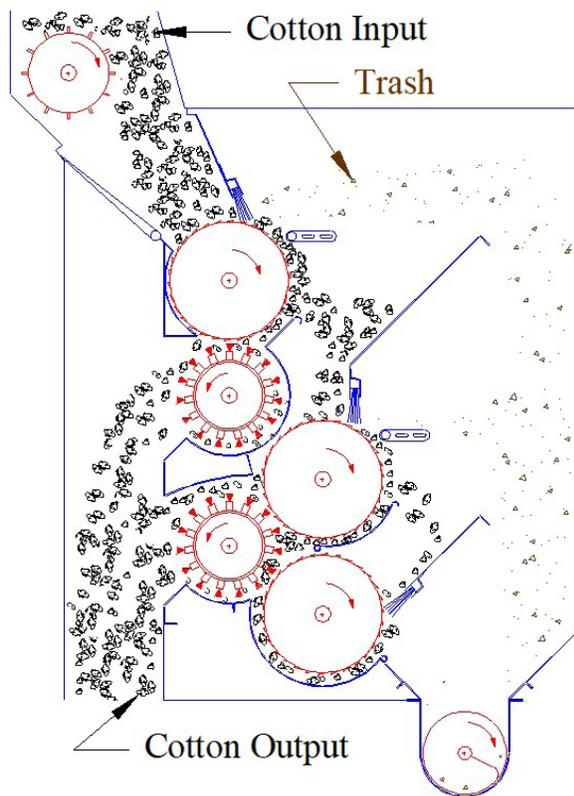
Figure 21. Three-saw stick machine (Armijo et al., 2009).
