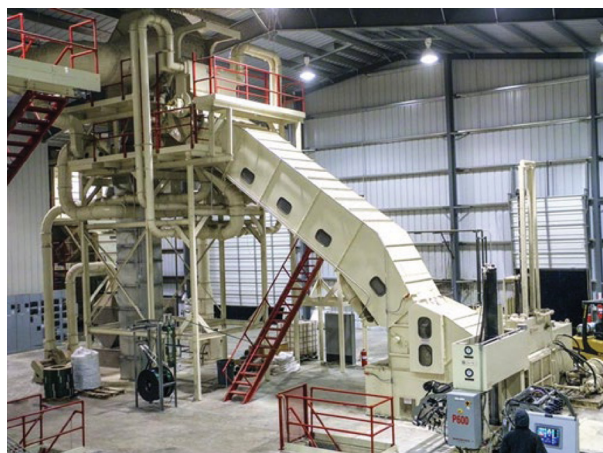
Figure 2. Fixed-Box bale press (courtesy of Cherokee Fabrication).
