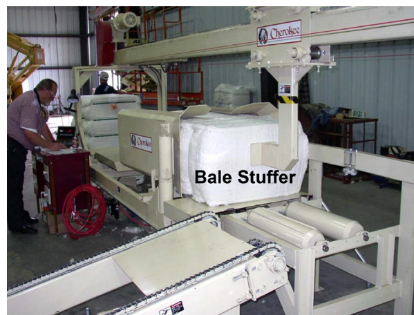
Figure 13. Bale stuffer system (courtesy of Cherokee Fabrication).
