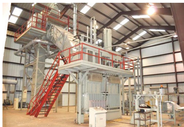
Figure 1. Down-packing bale press (courtesy of Lummus AG).
