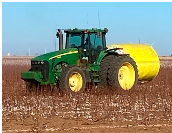
Figure 5. Transporting a module via multi-spike or smooth-fork implement attached to the three-point hitch of a tractor.
