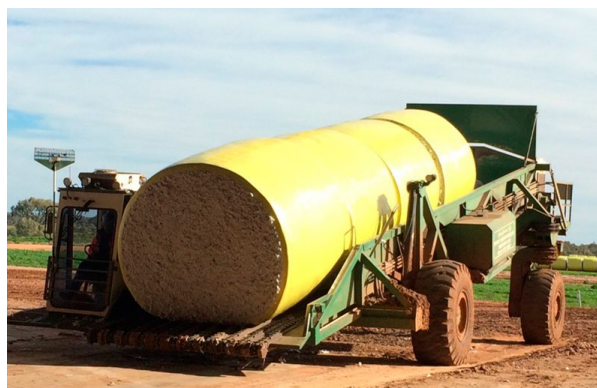
Figure 8. Typical Australian moon buggy transporting modules on the gin yard in sausage orientation.
