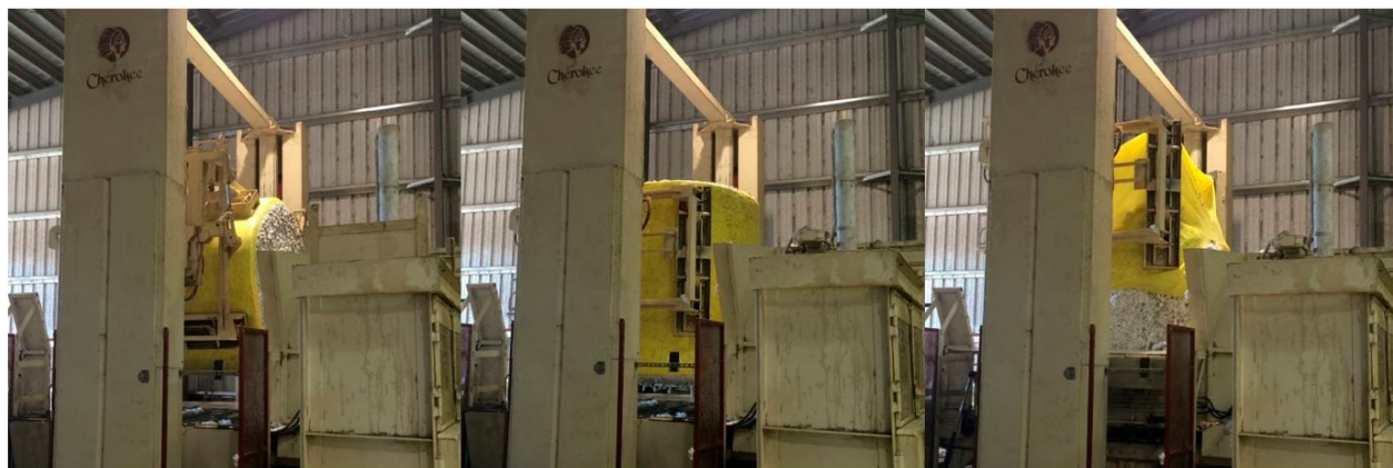
(a) Lifting the sausage style module (b) Module rotated to vertical (c) Seed Cotton sliding out of wrap Figure 13. Cherokee Round-Up Module Unwrapper.
