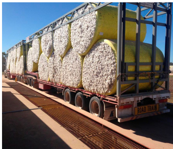
Figure 6. CM Cotton Cartage trailer with 18-module capacity.
