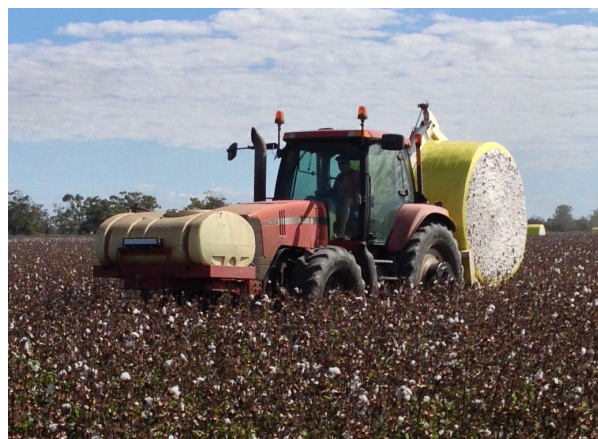
Figure 4. Mast-type tractor mounted implement that holds the module with the axis parallel to the tractor rear axle.
