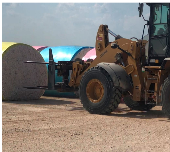
Figure 7. Front-end loader equipped with spikes for handling modules.
