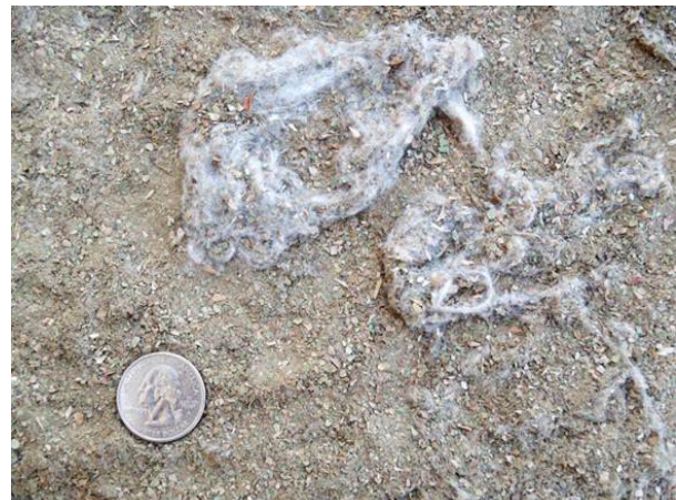
Figure 3. Photograph of typical trash captured by the unloading system cyclones.
