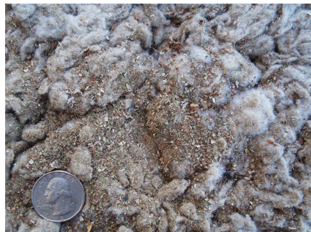
Figure 3. Photograph of typical trash captured by the mote trash system cyclones.
