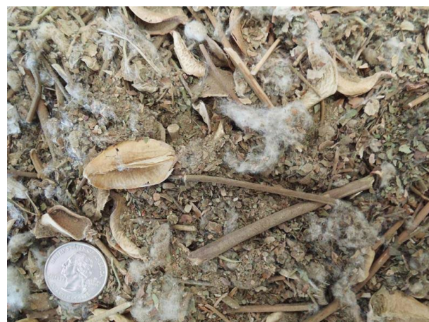
Figure 3. Photograph of typical trash captured by the master trash system cyclones.
