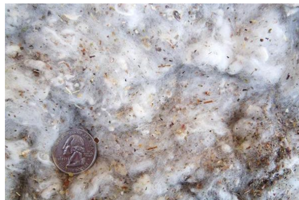
Figure 3. Photograph of typical trash captured by the mote cyclone robber system cyclones.
