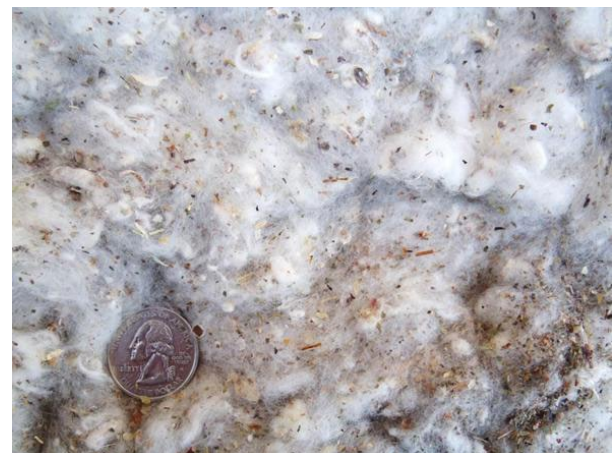
Figure 3. Photograph of typical trash captured by the combined mote system cyclones.
