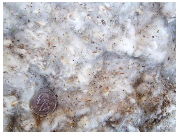
Figure 3. Photograph of typical trash captured by the 1 st stage mote system cyclones.
