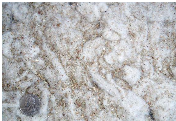
Figure 3. Photograph of typical trash captured by the 1 st stage lint cleaning system cyclones.
