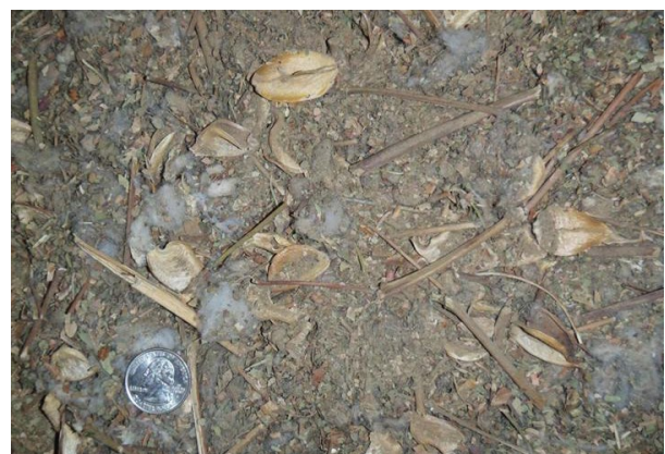
Figure 3. Photograph of typical trash captured by the 3 rd stage seed-cotton cleaning system cyclones.
