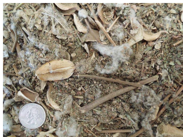
Figure 3. Photograph of typical trash captured by the 1 st stage seed-cotton cleaning system cyclones.
