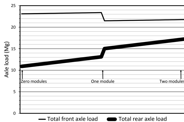
Figure 5. Dynamic axle loads for front and rear axles of a round baler cotton picker. The x-axis represents the time that takes to form a round bale. The space between these points is the transition phase as a bale is produced.
