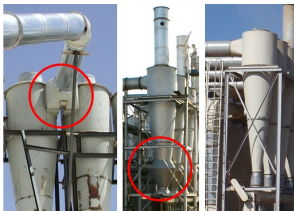
Figure 11. Cyclone design variations for the tested systems (left to right): dual configuration that splits flow between identical 1D3D cyclones with 2D2D inlets; 1D3D cyclone with 2D2D inlet and expansion chamber on the cone; 1D3D cyclone with 2D2D inlet and standard cone.
