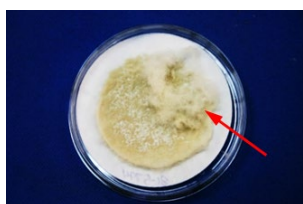
Figure 13. EPA Method 17 filter from the 2 nd stage lint cleaning system with lint on the filter (indicated by arrow).
