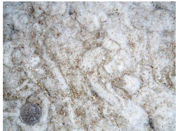
Figure 4. Photograph of typical trash captured by the 1 st stage lint cleaning cyclones.
