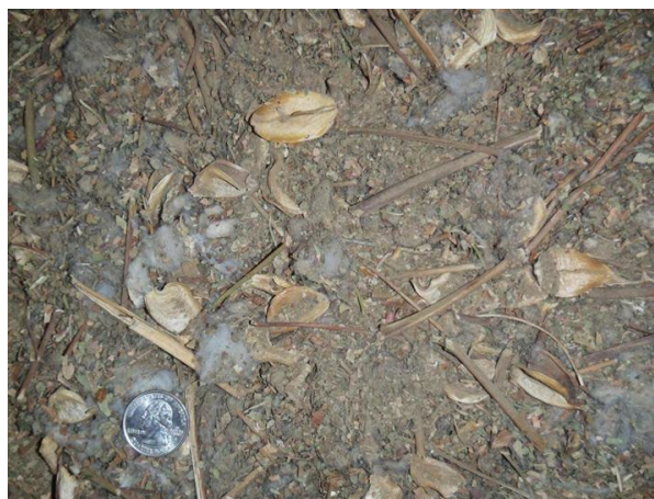
Figure 4. Photograph of typical trash captured by the 3 rd stage seed-cotton cleaning system cyclones.
