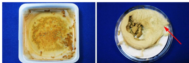
Figure 12. Typical EPA Method 17 filter and sampler head acetone wash from the mote cleaner system with lint fiber on the filter (indicated by arrow). From left to right: front half wash and filter.
