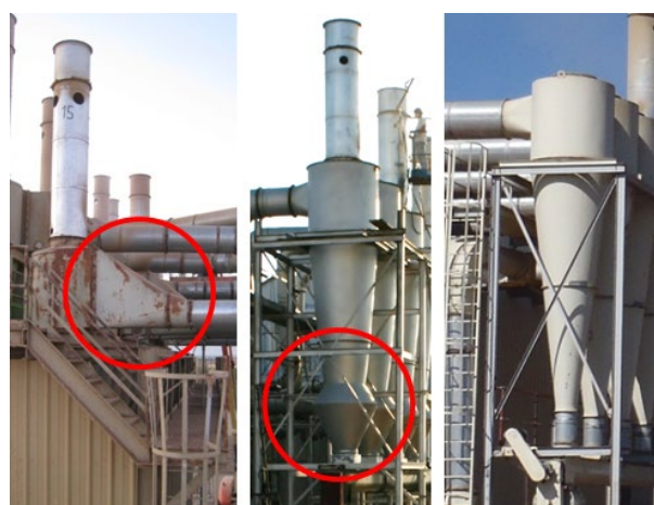
Figure 11. Cyclone design variations for the tested systems (left to right): 1D3D cyclone with an inverted 1D3D inlet; 1D3D cyclone with 2D2D inlet and expansion chamber on the cone; 1D3D cyclone with 2D2D inlet and standard cone.
