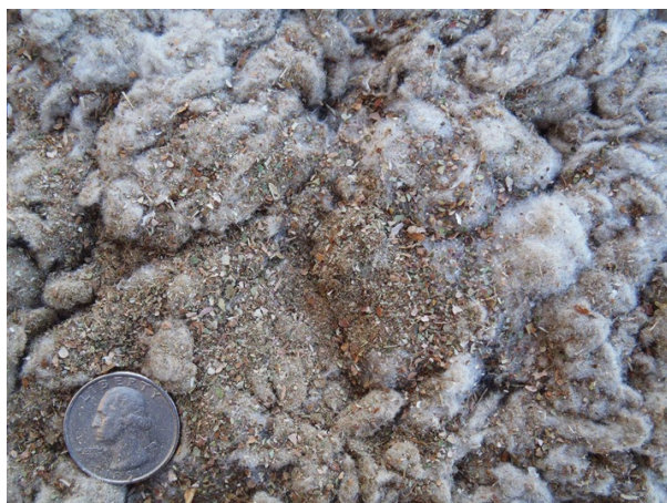
Figure 4. Photograph of typical trash captured by the mote trash system cyclones.
