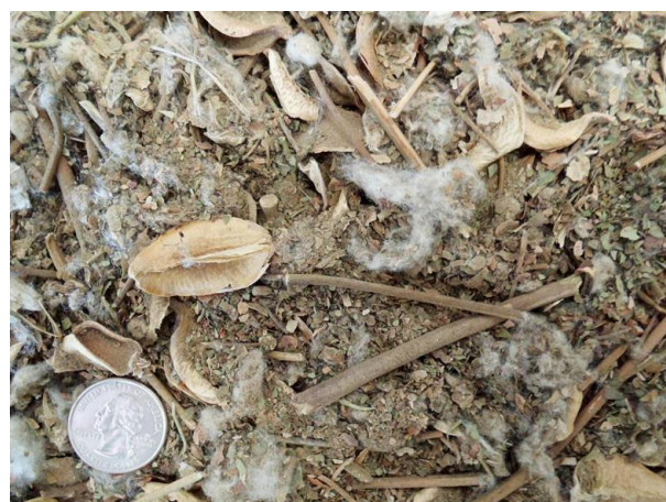
Figure 4. Photograph of typical trash captured by the master trash system cyclones.
