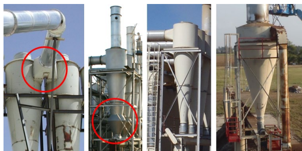
Figure 9. Cyclone design variations for the tested systems (left to right): dual configuration that splits flow between identical 1D3D cyclones with 2D2D inlets; 1D3D cyclone with 2D2D inlet and expansion chamber on the cone; 1D3D cyclone with 2D2D inlet and standard cone; \frac{1}{2} D2D cyclone with a square inlet measuring about \frac{1}{4} D on a side.
