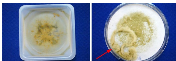
Figure 12. Typical EPA Method 17 filter and sampler head acetone wash from the mote cyclone robber system with lint on the filter (indicated by arrow). From left to right: front half wash and filter.
