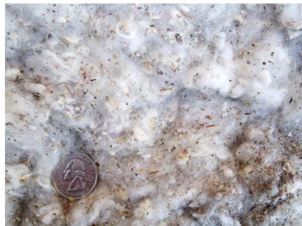
Figure 4. Photograph of typical trash captured by the mote cyclone robber system cyclones.
