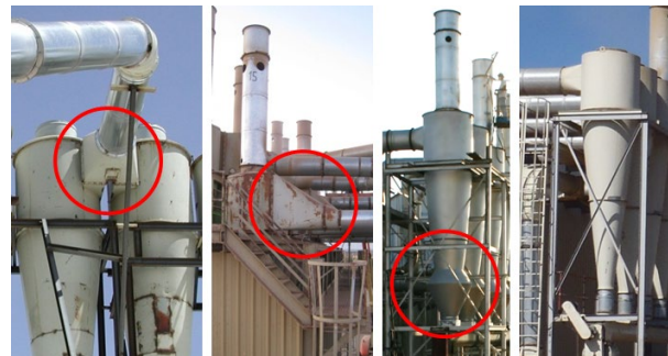
Figure 13. Cyclone design variations for the tested systems (left to right): dual configuration that splits flow between identical 1D3D cyclones with 2D2D inlets; 1D3D cyclone with an inverted 1D3D inlet; 1D3D cyclone with 2D2D inlet and expansion chamber on the cone; 1D3D cyclone with 2D2D inlet and standard cone.
