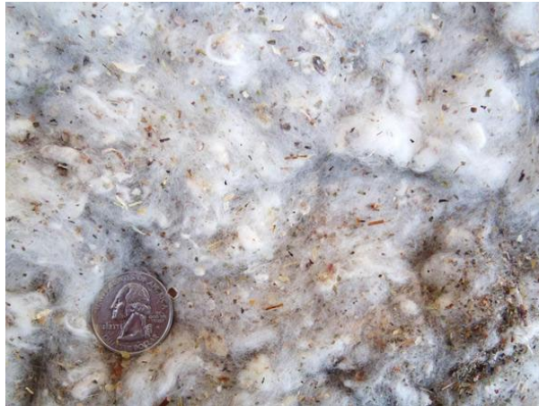
Figure 4. Photograph of typical trash captured by the second stage mote system cyclones.
