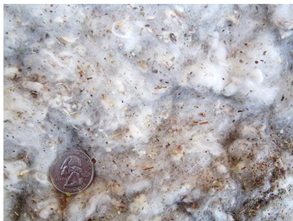
Figure 4. Photograph of typical trash captured by the first stage mote cyclones.
