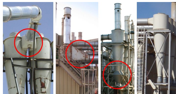
Figure 13. Cyclone design variations for the tested systems (left to right): dual configuration that splits flow between identical 1D3D cyclones with 2D2D inlets; 1D3D cyclone with an inverted 1D3D inlet; 1D3D cyclone with 2D2D inlet and expansion chamber on the cone; 1D3D cyclone with 2D2D inlet and standard cone.
