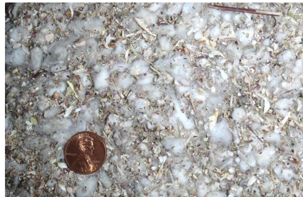
Figure 4. Photograph of typical trash captured by the mote trash system cyclones.
