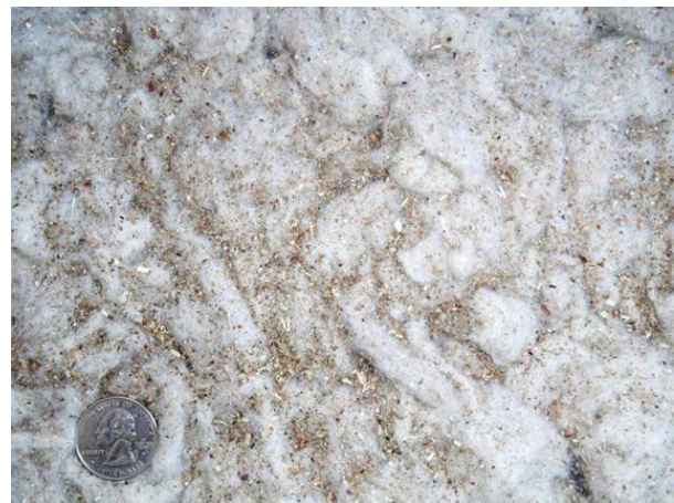
Figure 4. Photograph of typical trash captured by the combined lint cleaning system cyclones.
