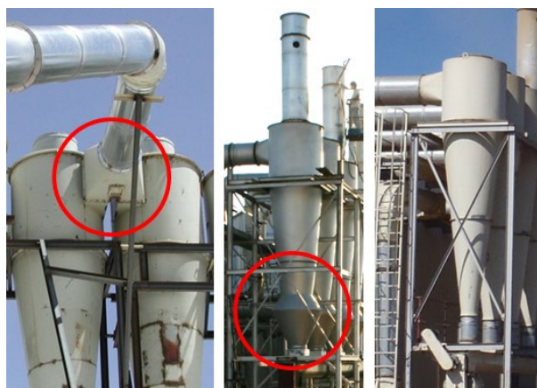
Figure 12. Cyclone design variations for the tested systems (left to right): dual configuration that splits flow between identical 1D3D cyclones with 2D2D inlets; 1D3D cyclone with 2D2D inlet and expansion chamber on the cone; 1D3D cyclone with 2D2D inlet and standard cone.
