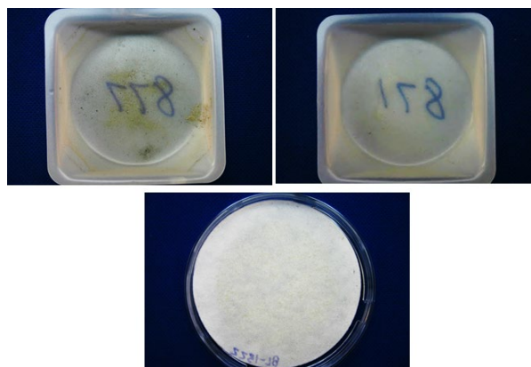
Figure 13. Typical EPA Method 201A filter and sampler head acetone washes from the 2 nd stage lint cleaning. Clockwise from top left: > 10 μm wash, ≤ 10 μm wash and filter.
