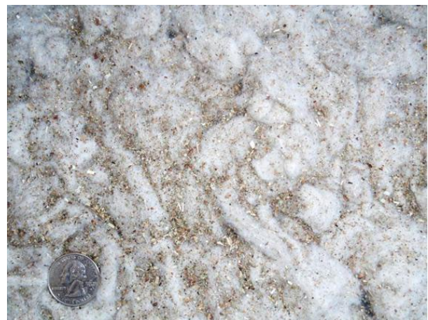
Figure 4. Photograph of typical trash captured by the 2 nd stage lint cleaning system cyclones.
