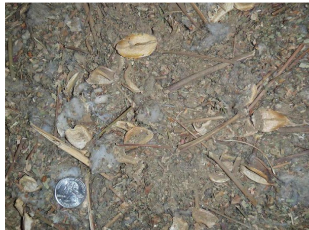
Figure 4. Photograph of typical trash captured by the 3 rd stage seed-cotton cleaning system cyclones.
