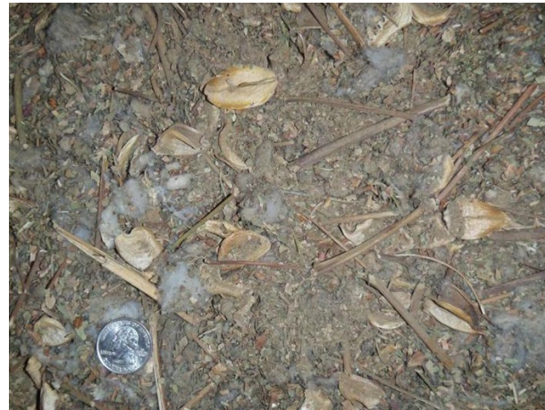
Figure 4. Photograph of typical trash captured by the 2 nd stage seed-cotton cleaning system cyclones.
