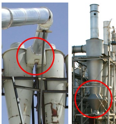
Figure 12. Cyclone design variations for the tested systems (left to right): dual configuration that splits flow between identical 1D3D cyclones with 2D2D inlets; 1D3D cyclone with 2D2D inlet and expansion chamber on the cone.
