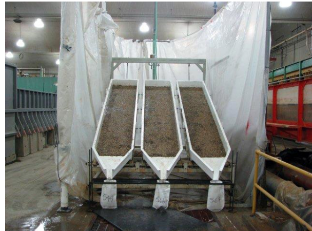
Figure 2. Triplicate soil plot test configuration. Soil trays on soil cart elevated at 2H:1V.
