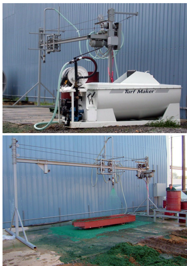
Figure 1. Hydromulcher with application gantry system in background (top) and gantry system applying uniform treatment application rate on soil tray (bottom).
