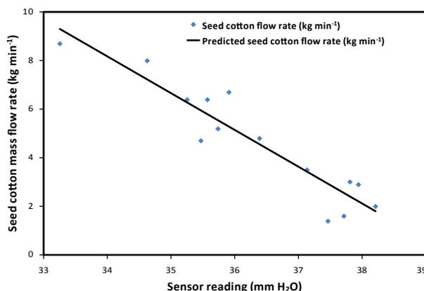
**Figure 5.** Relationship between air velocity pressure and seed cotton mass flow rate for wet cotton.
