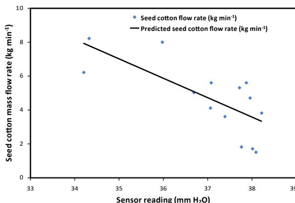
**Figure 4.** Relationship between air velocity pressure and seed cotton mass flow rate for dry cotton.
