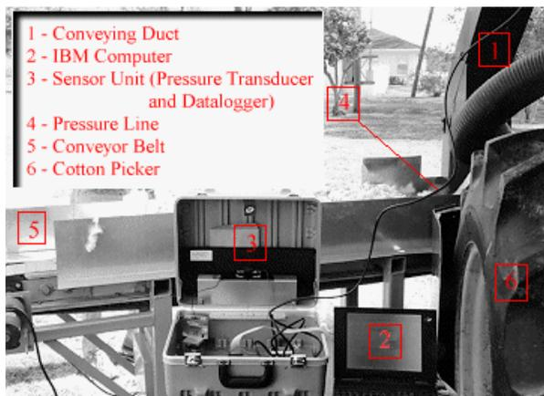
Figure 2. Cotton-picker testing equipment.
