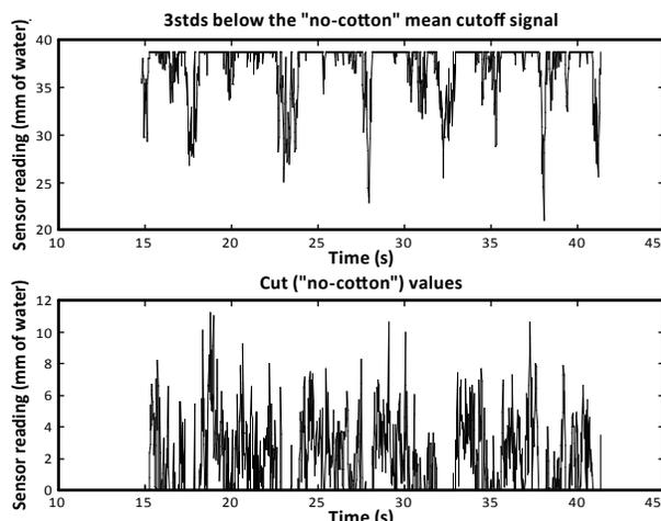
**Figure 3.** Sensor signal profile for compensated no-cotton gaps (top) and eliminated background noise signal while no cotton is being transported for the 7.7 kg min<sup>-1</sup> dry cotton (bottom).
