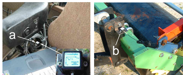
Figure 3. Placement of one-dimensional (z-axis) accelerometer from Crossbow Technology: (a) tractor's frame, and (b) roller's frame.
