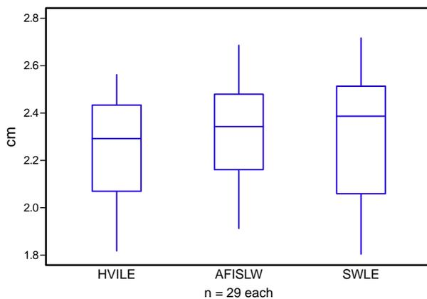
**Figure 3. Box-and-whisker plots indicating the distribution of mean fiber lengths measured by HVI, AFIS, and Suter-Webb array.**
