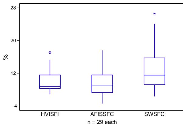
**Figure 1. Box-and-whisker plots indicating the distribution of short fiber contents measured by HVI, AFIS, and Suter-Webb array.**
