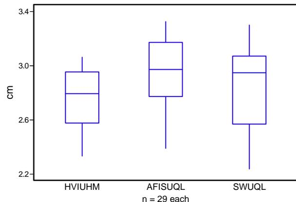
**Figure 5. Box-and-whisker plots indicating the distribution of long fiber lengths measured by HVI, AFIS, and Suter-Webb array.**
