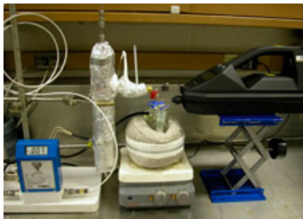
Figure 2b. IMS sensing vapors from a heated flask containing plastic and cotton. Left to Right: gas mass flow meter, pure air preheater, 500 ml flask on hot plate, and IMS representative of analyzers used in these trials.
