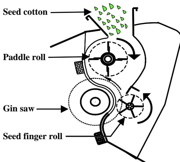
Figure 1. Schematic cutaway view of the powered roll gin stand showing the location of the paddle roll and seed finger roll relative to the gin saw.
