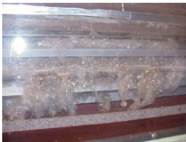
Figure 5. Waste emitted from the experimental lint cleaner during operation at Stoneville.
