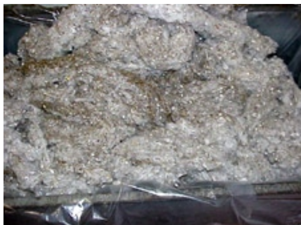
Figure 3. Typical waste from a Sixteen D lint cleaner.
