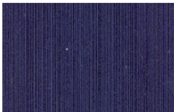
Figure 2. An example of white specks on a yarn board.
