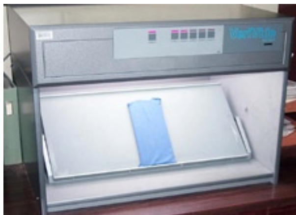
Figure 1. Leslie Hubble Ltd. VeriVide Model CAC 60-5 Light Cabinet used by the operators in counting white specks.
