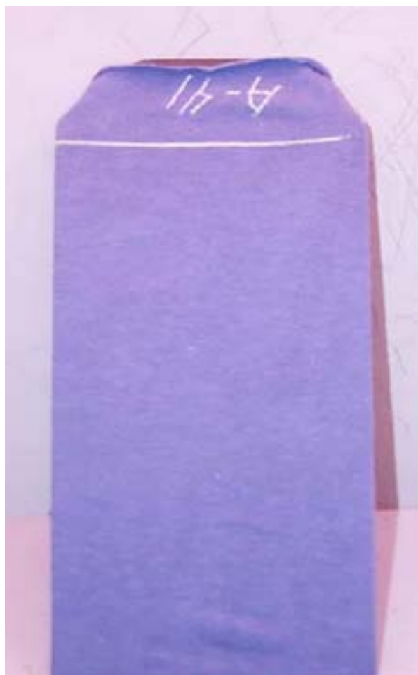
Figure 3. FAK knit tube sample loaded on a template for viewing white specks.
