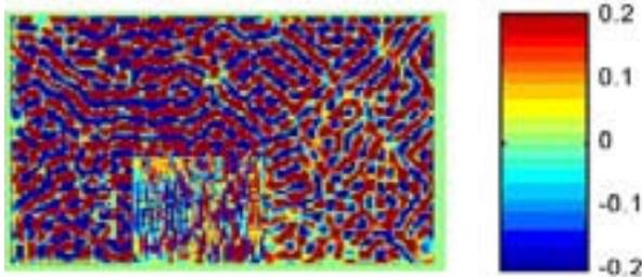
Figure 10: Steady state solution of a wet bale in a metal clad building. The colors are the relative range of signal strength (H/m).
