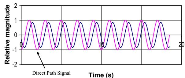
**Figure 1:** Comparison of a direct-path signal (pink signal with the peak to peak magnitude = 2) with the combination of the direct-path signal with two multipath delayed signals of differing amplitudes and phases.
