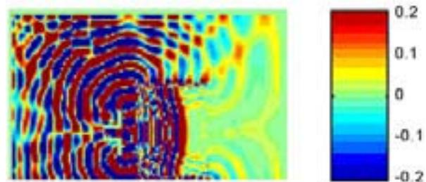
**Figure 6: Transient response of a wet bale inside a metal structure. The colors are the relative range of signal strength (H/m).**
