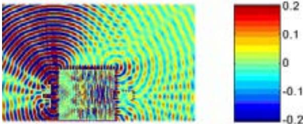
Figure 8: Steady state solution of a wet bale in free space. The colors are the relative range of signal strength (H/m).
