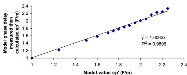
**Figure 5: Results of the correlation analysis between the closed form solution to Maxwell's equations for a plane-wave and successful prediction of the permittivity ( $\epsilon_p'$ ) of a dielectric absorber by the finite-difference time-domain (FDTD) model.**
