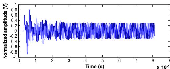
**Figure 3:** All of the finite-difference time-domain (FDTD) simulations were run until steady state conditions were observed. The y axis is relative magnitude of the received signal strength and the x axis is time in seconds. The permittivity was calculated for all of the simulations by using only data that was obtained after steady state conditions were achieved. In this case, the signal was assumed to be stable after  $4e-8$  seconds.
