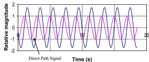
**Figure 2:** Comparison of a direct-path signal (pink signal with the peak to peak magnitude = 2) with the combination of the direct-path signal with a different set of two multipath delayed signals of differing amplitudes and phases.
