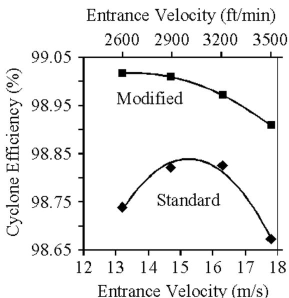
**Figure 2. Plot of cyclone efficiency vs. entrance air velocity for standard design and average of all three modified designs.**
