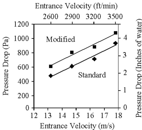
**Figure 3. Plot of cyclone pressure drop vs. entrance air velocity for standard design and average of all three modified designs.**
