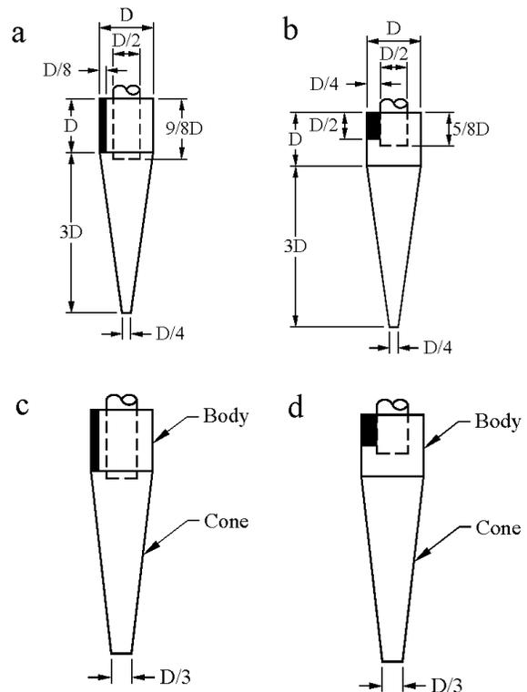
**Figure 1.** 1D3D cyclones of diameter  $D$  including a) standard entrance ( $D/8$  wide), standard trash outlet ( $D/4$ ); b) modified entrance ( $D/4$  wide), standard trash outlet ( $D/4$ ); c) standard entrance ( $D/8$  wide), modified trash outlet ( $D/3$ ); d) modified entrance ( $D/4$  wide), modified trash outlet ( $D/3$ ).
