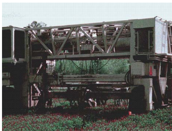
Figure 1. Wide-Frame Tractive Vehicle used at the USDA-ARS National Soil Dynamics Laboratory to study the effects of traffic-free zones on soil compaction.
