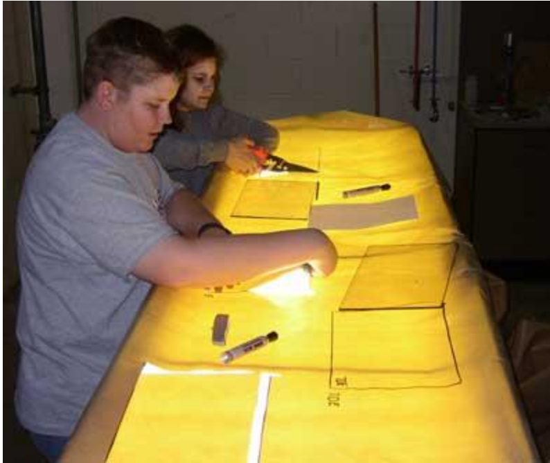
Texas A&M University researchers inspect new and used module covers on a light table and categorize them based on condition prior to cutting samples for water penetration tests.
