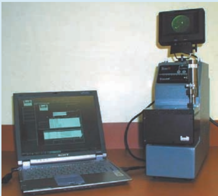
An infrared instrument and a laptop computer are used to identify cotton trash particles based on unique wavelength signatures.
