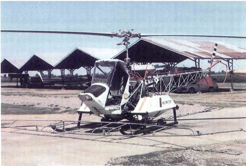
Figure 23. Continental Copter, Mark 5 Tom Cat, equipped with Warner spray system nozzles.
