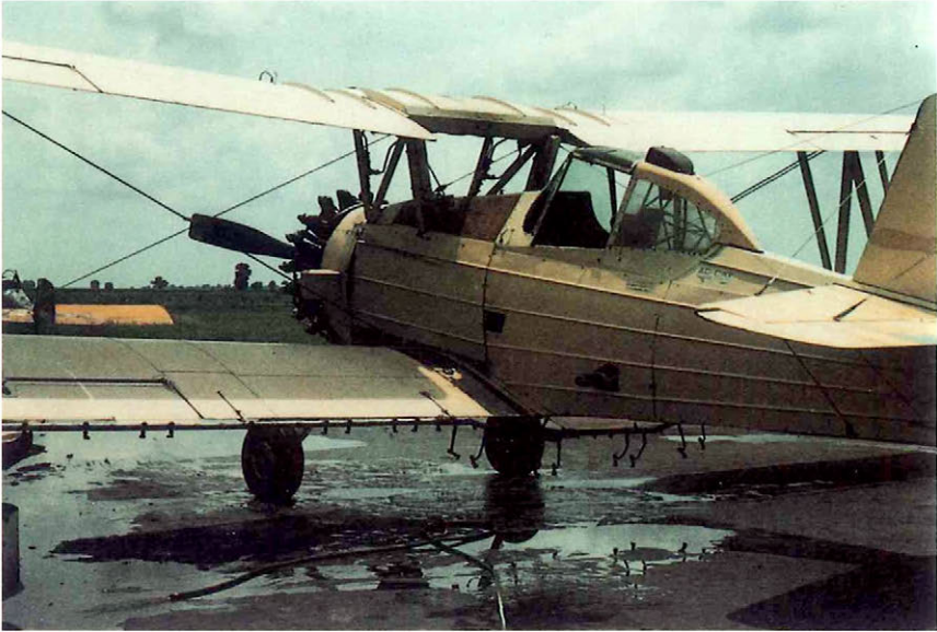
Figure 20. Gruman G-164B Ag-Cat equipped with combination nozzles.
