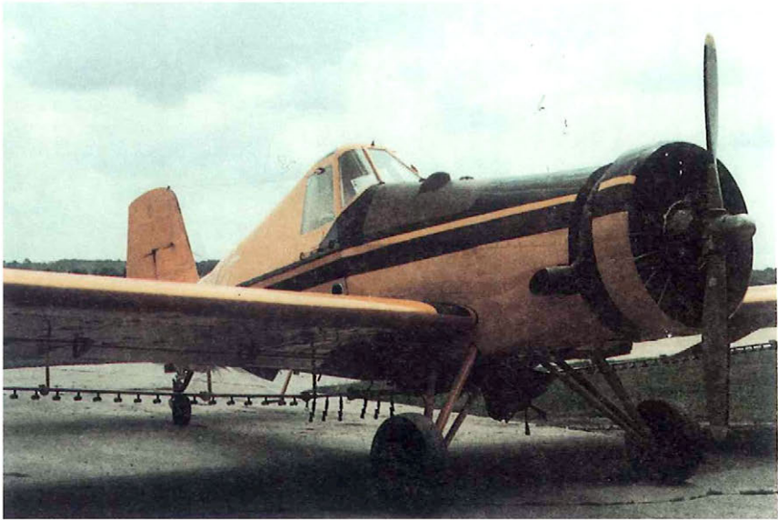
Figure 18. Rockwell Thrush Commander 600 equipped with combination nozzles.
