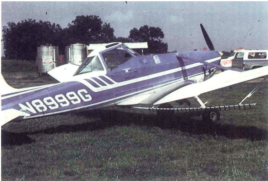
Figure 15. Cessna A188B Ag-Wagon equipped with combination nozzles.
