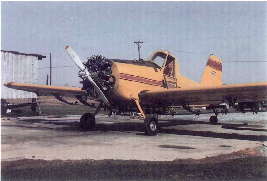
Figure 21. Air Tractor AT-301, 600, equipped with Model 10 Unimizer spinning atomizers.
