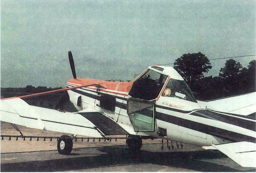
Figure 16. Cessna A188B Ag-Husky-Turbo equipped with combination nozzles.
