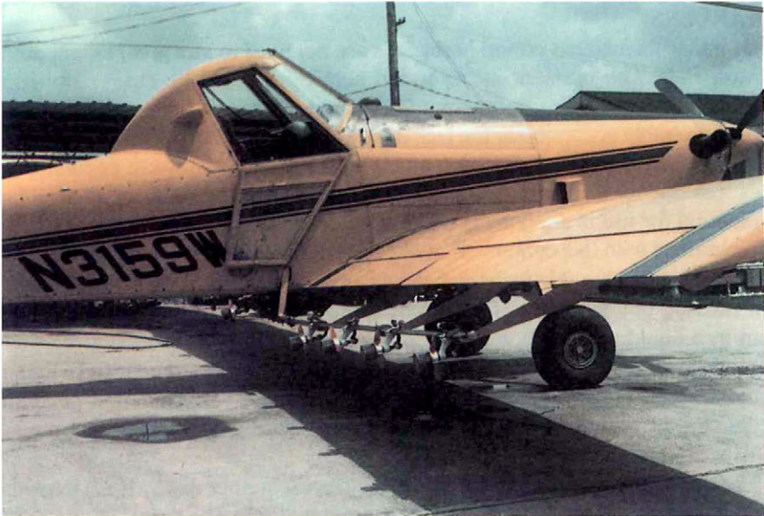
Figure 22. Air Tractor AT-301, Turbo 680, equipped with Micronair spinning atomizers.
