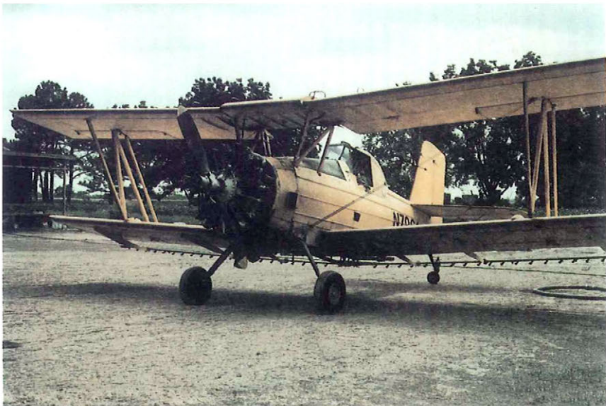
Figure 19. Gruman G-164A Ag-Cat equipped with combination nozzles.
