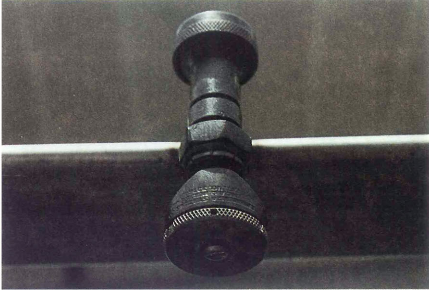
Figure 13. A combination pressure nozzle used on aircraft.
