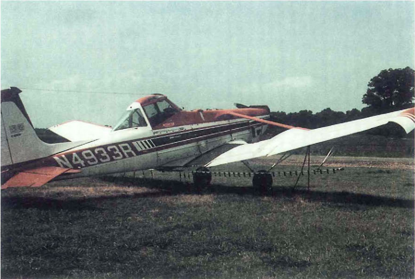
Figure 17. Cessna A188B Ag-Truck equipped with combination nozzles.
