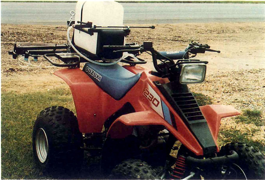
Figure 11. One of several types of all terrain vehicles equipped with a sprayer which can be used for spot-spraying.
