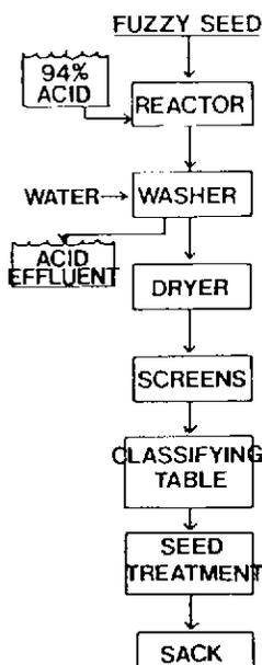
Figure 9. Generalized flow chart for the conventional wet-acid delinting process for cottonseed (from Jones, (1980).
