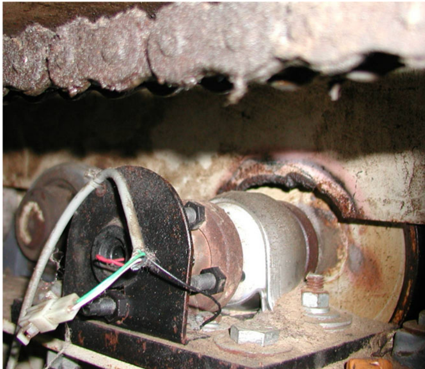
Figure 2. Photograph of the installation at the end of one roller showing the roller, pillow block, proximity switch and two magnets, and electrical connections including the end of the slip ring.
