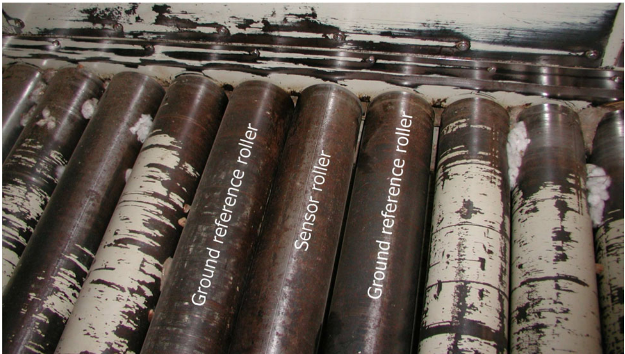
Figure 3. Photograph of the measurement roller and the two adjacent ground reference rollers with the paint removed.
